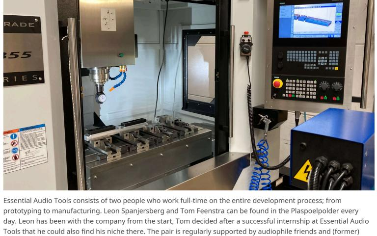
Our own disciplines are sufficient to design products on computer screens via Computer Aided Design and rendering software. To then produce parts on an inhouse CNC machine. When a product is ready for production, the machine is programmed to make series.
